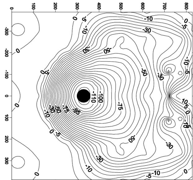
Fig. 4 Scour pattern around a pier without countermeasure
