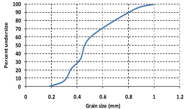
Figure 2. Grain size distribution curve of the sediment used in tests.
