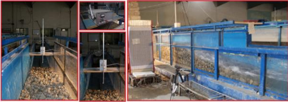
Figure 2. Profile indicator to recording the geometry of the barrier
