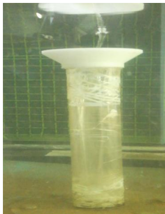
Figure 5. Bell-mouth vertical intake used in present work.
