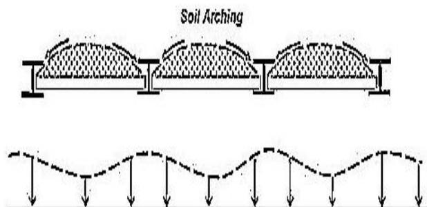
**Figure 2.** Soil arching between piles
