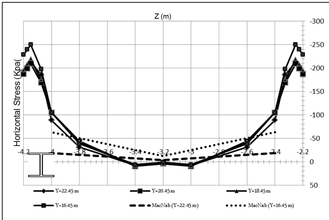
**Figure 6.** Horizontal stress distribution ( $\sigma_{xx}$ ) in different depths between two piles with axial distance 2 m
