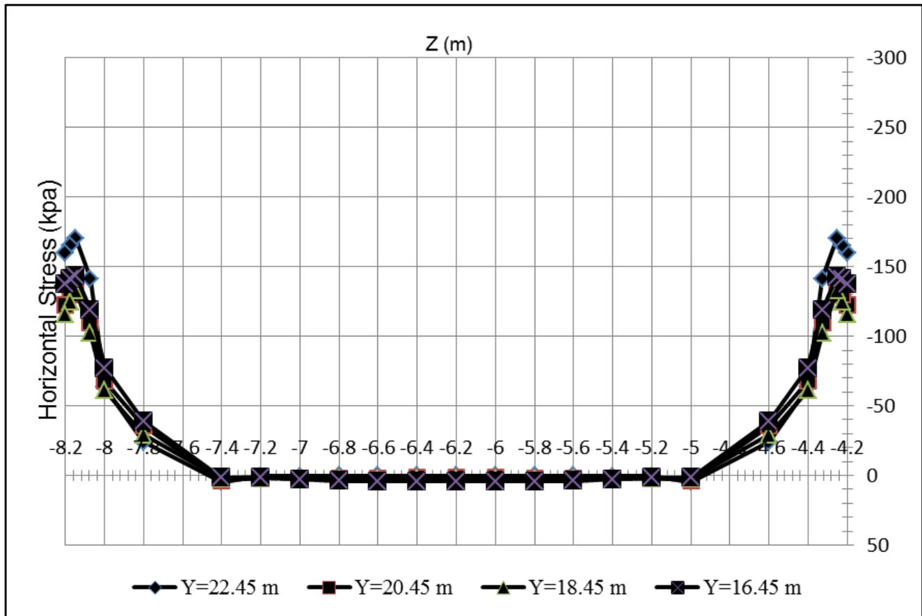
Figure 7. Horizontal stress distribution ( $\sigma_{xx}$ ) in different depths between two piles with axial distance 4 m
