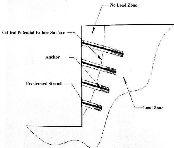
**Figure 3.** Load zone and no load zone in anchorage method
