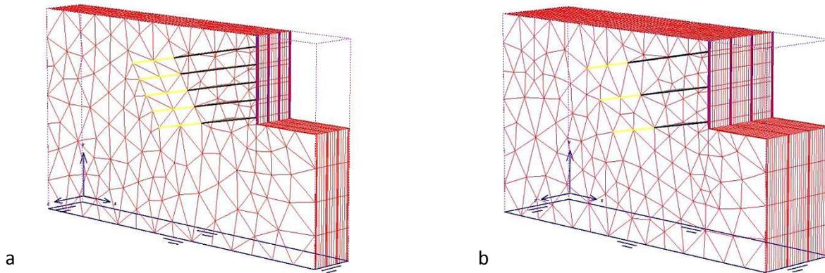
**Figure 5.** Final excavation phase: a) 2m distance between piles; b) 4m distance between piles
