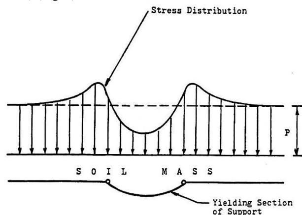
**Figure 1.** Stress distribution in the soil above a yielding base (Bjerrum et. al., 1972; Revised by Evans, 1984)
