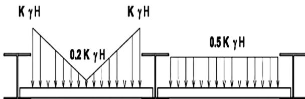
Figure 8. Diagrams reduced pressure on board between two piles
