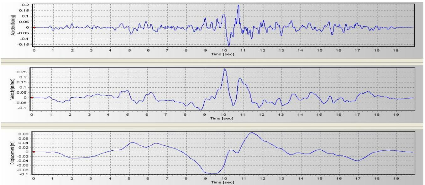
Figure 8. Earthquake accelerograms, velocity, and displacement of Spitak earthquake
