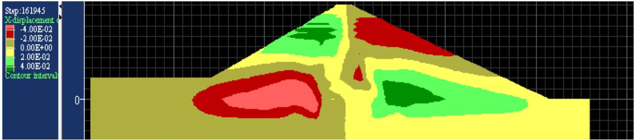
Figure 3. Horizontal deformation after construction
