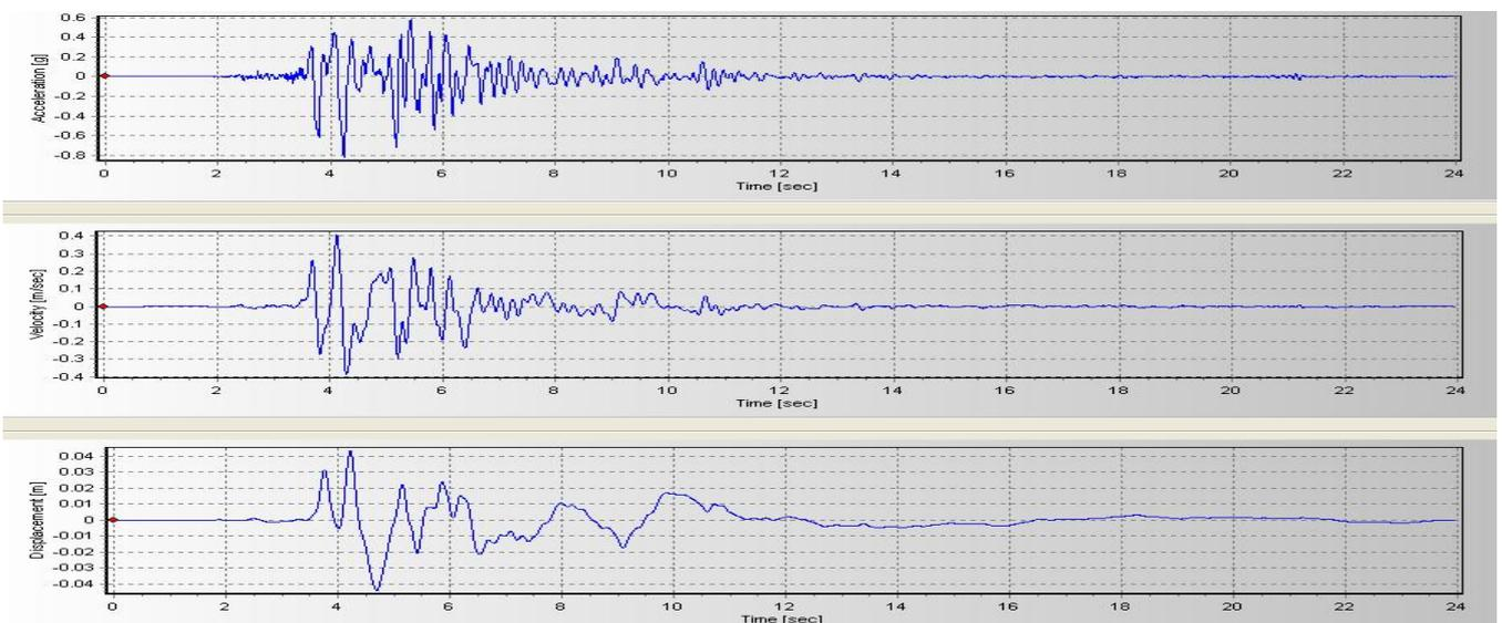
Figure 9. Earthquake accelerograms, velocity, and displacement of Kobe earthquake
