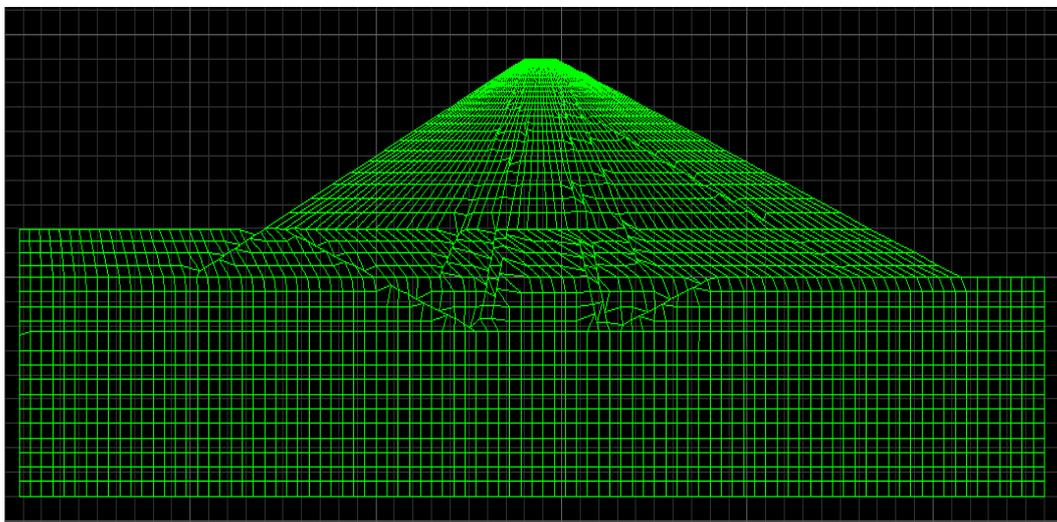
Figure 1. Finite Difference Network for EMARAT earth dam
