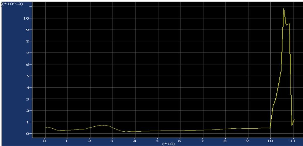
Figure 19. Diagram of shear strain in the dam due to Kobe earthquake
