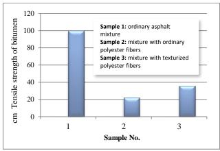
Graph 1. The test results of tensile strength
